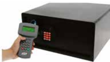
Emergency opening Prolog Service Unit (PSU)
